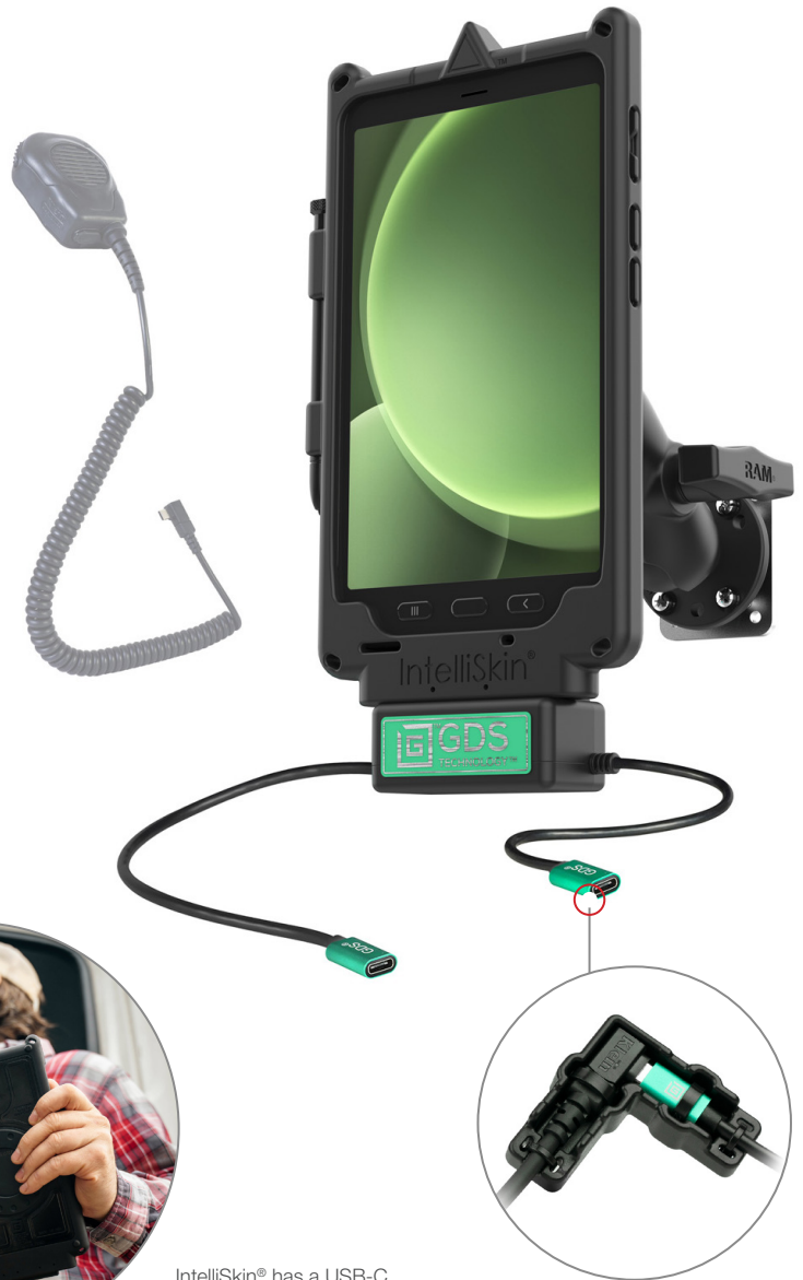
IntelliSkin® has a USB-C port so that workers can plug their microphone in as needed
