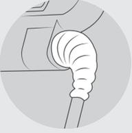
Oversized strain relief protects cable connection
