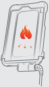
Open enclosure on front and back allows heat to flow from device.
