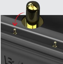
When connected to a power source, two integrated pogo pins provide charging capabilities to the device
