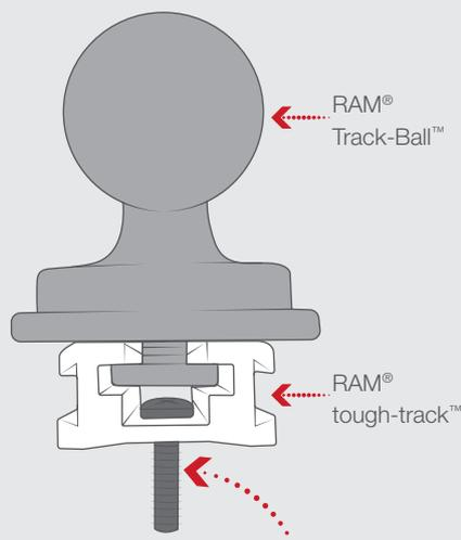
RAM® Tough-Track™ can be drilled to any flat surface and is designed for use with #8 screws for easy installation – hardware not included
