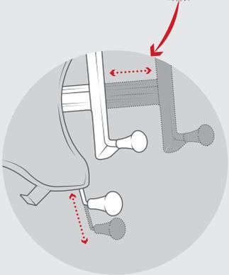
Additional grip handles for convenient insertion and removal
