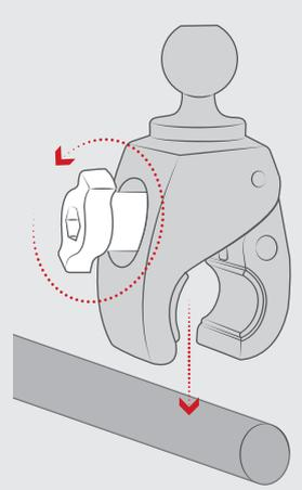
Toolless installation for convenient installation, transfer and removal of base
