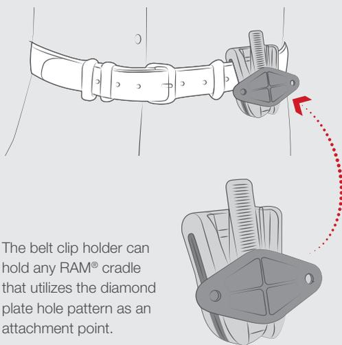
The belt clip holder can hold any RAM® cradle that utilizes the diamond plate hole pattern as an attachment point.
