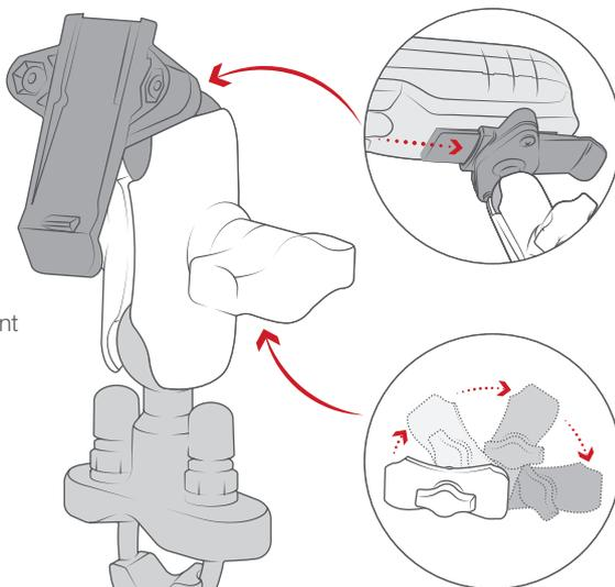
Holder secures any Garmin handheld device with an integrated spine connection
