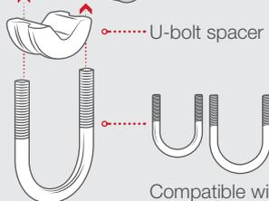
U-bolt spacer protects handlebar surface
