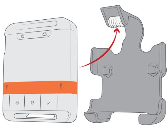
Simply slide your SPOT Gen4™ into the cradle and roll the top clip over the device to secure into place.
