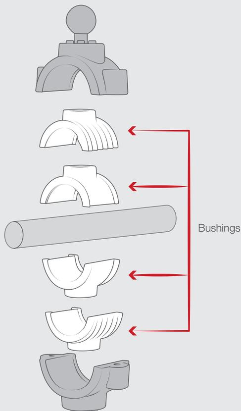
Internal bushings conform to your handlebar while protecting the surface
