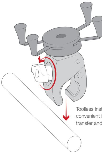
Toolless installation for convenient installation, transfer and removal of base
