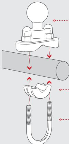
1" rubber ball is designed to sit at right angles to mounting rail
