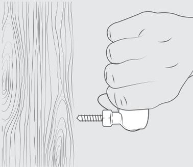
Grab onto Socket Arm and 1/4"-20 Ball and position self-tapping threads against desired mounting point.
