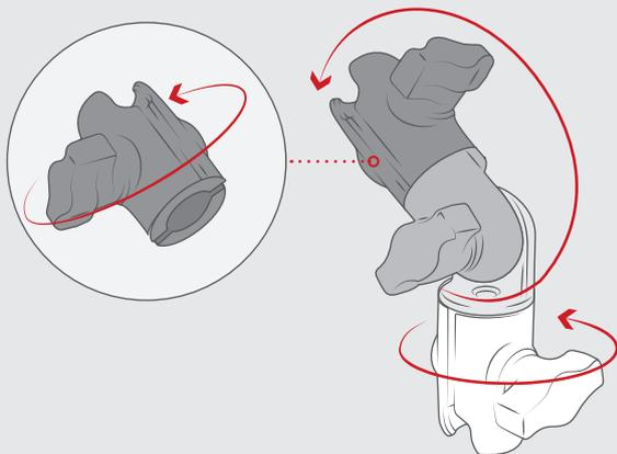
Double socket swivel and ratchet arm features 360-degree center rotation and 180-degree swivel joint allowing for near-infinite adjustability of your RAM® mounting system
