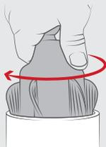
Insert and twist the Stubby™ into your cup holder to create proper friction.
