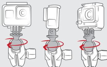
Adjustable position of camera with the turn of a single knob
