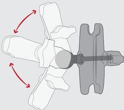
The RAM-B-273U allows for connection to any B size RAM® double socket arm; ball and socket technology allows for near-infinite adjustability
